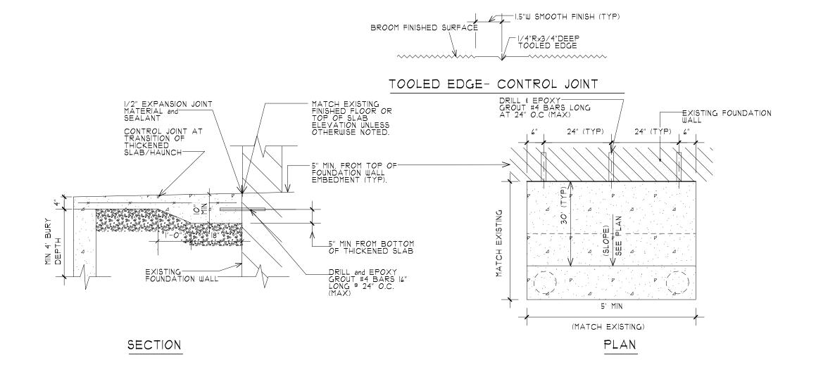
3 CONCRETE SIDEWALK AT BUILDING ENTRANCE AZ SCALE: NOT TO SCALE
