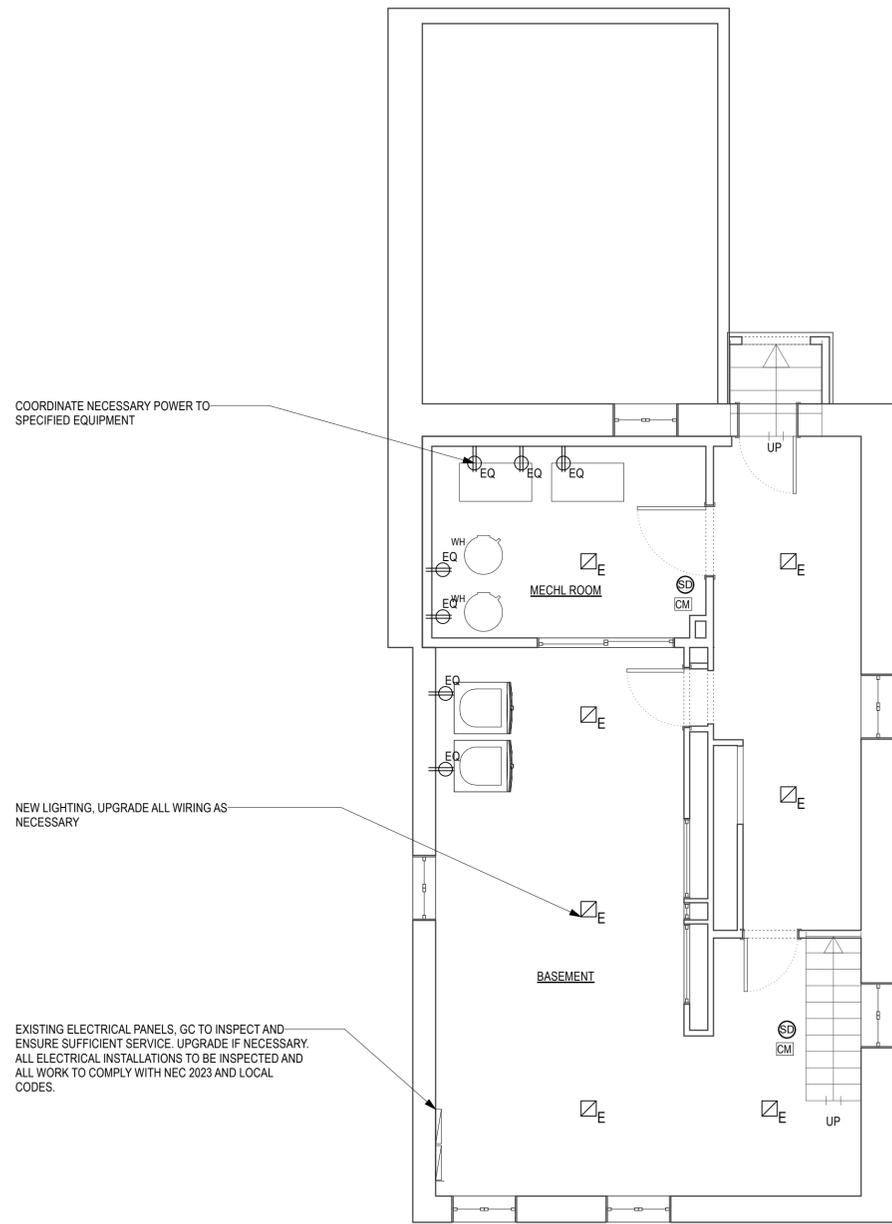
COORDINATE NECESSARY POWER TO SPECIFIED EQUIPMENT
